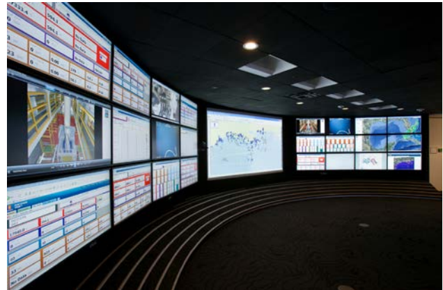
Fig. 4 The data wall is a highly visible, public display providing a dashboard view of the GoM drilling and completion operations.
